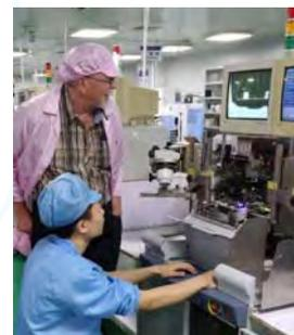
In between each pass of the P&P machine, you have to manually change the LED chip holders to the next set, before restarting the P&P machine - another time and labour intensive operation.
