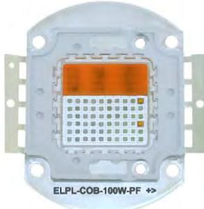
The EconoLux ELPL-COB-100W-PF, 24 band, LED grow light-engine is our LED COB (Chip On Board) with a 95% match to the PAR curve, with about 10% extra Red light. It produces 333.6 PAR/PPFD\* at a distance of 30 cm (1 ft) - that's 3.36 PPFD/Watt!
