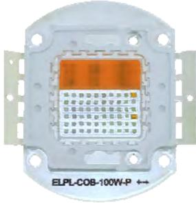
The EconoLux ELPL-COB-100W-P, 24 band, LED grow light-engine is our 100W, LED COB (Chip On Board) with a 90% match to the PAR curve. It produces 346.7 PAR/PPFD\* at a distance of 30 cm (1 ft) - that's 3.47 PPFD/Watt!
